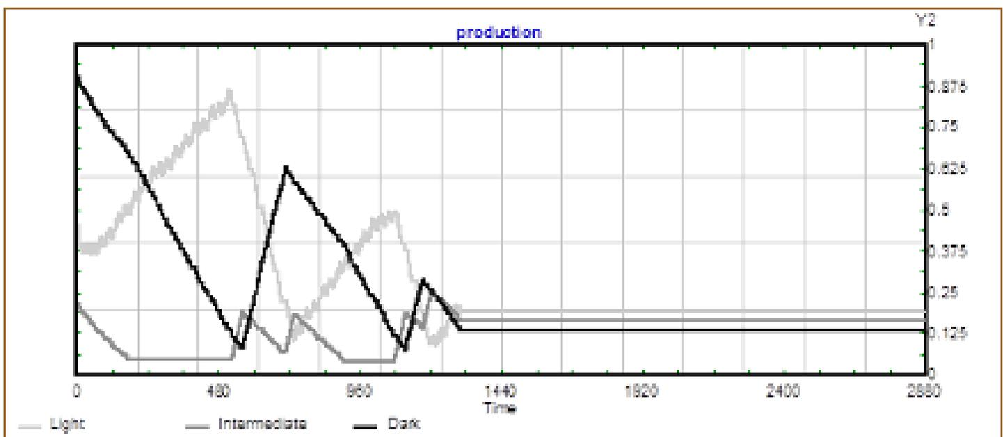
Figure 10. Low Yield Silo Inventory Agglomeration cannot fulfil downstream demand and Process shuts down due to low silo inventory.
