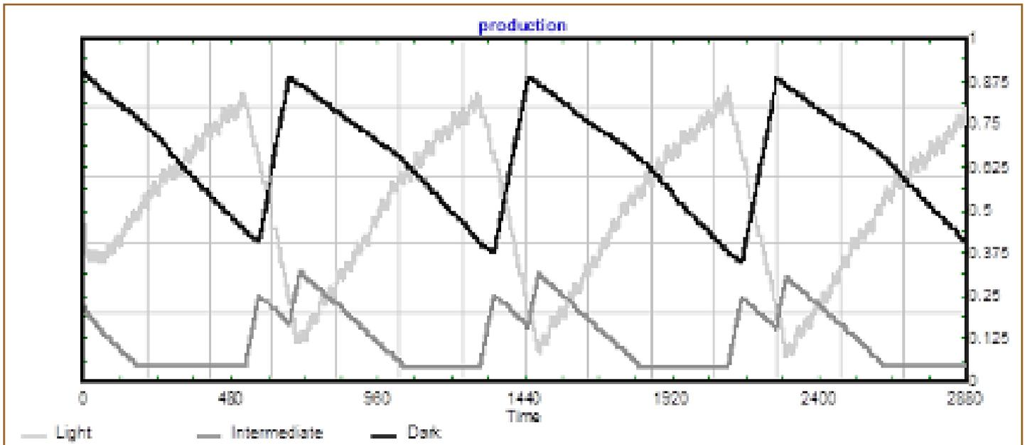
Figure 6. Silo Levels of agglomerated particles
