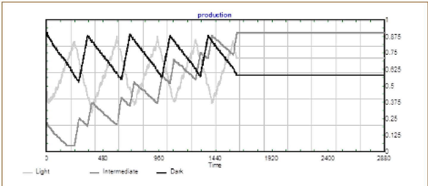
Figure 12. High Yield Silo Inventory: Agglomeration process exceeds downstream demand and overfills silo. Transition material is not managed.
