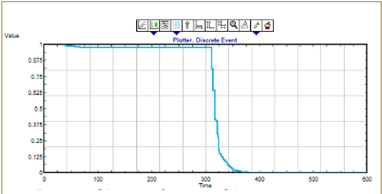
Figure 4. Dimensionless activated carbon level after recipe transition at 300 minutes.
