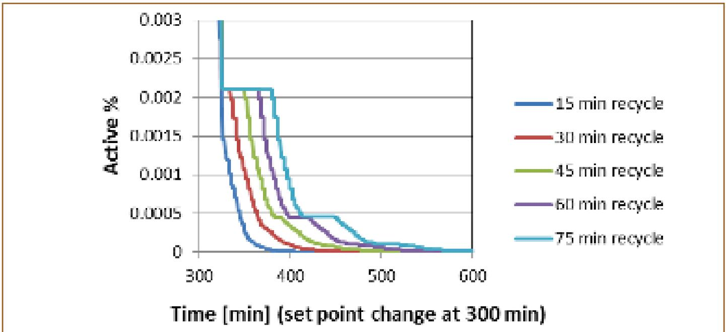
Figure 5. Transition time differences as a function of recycle level in recycle tank
