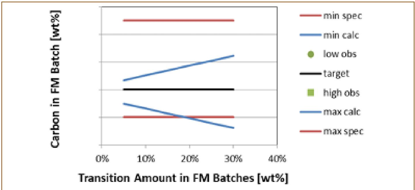
Figure 9. Carbon variability in finished product as a function of transition material added
