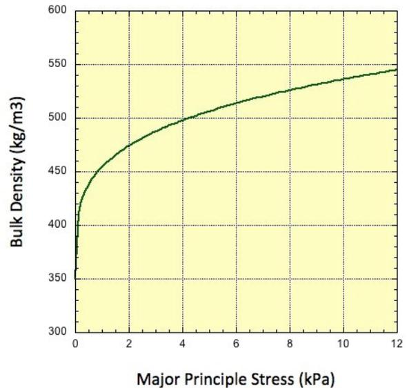
Figure 2. Compressibility of bulk solid.
